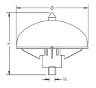
Material: Stainless Steel 316 (EN 1.4401) Temperature: -40 to 100 °C
